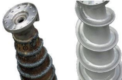
Repair parts (for example scroll restoration)
